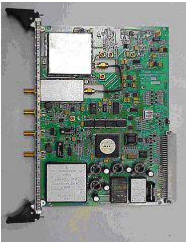
Dual channel impulse radar transceiver
