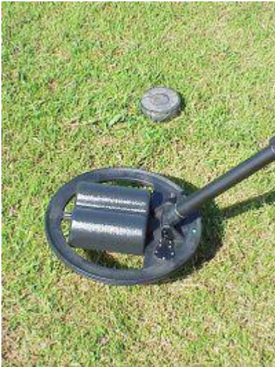
Sensor head of the Minetect hand held mine detection system
