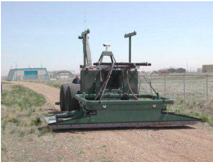
ERA multi-channel ground penetrating radar mounted on a specialist vehicle
